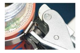
Roll hose over until shear hook engages behind buckle edge, at the same time reversing handle approx. half turn (depending on type and size of hose).
