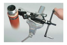
Insert hose into clamp and apply tension. To control tensioning, hold thumb on that side of buckle where band enters. When band stops moving through buckle, maximum tension has been applied.
